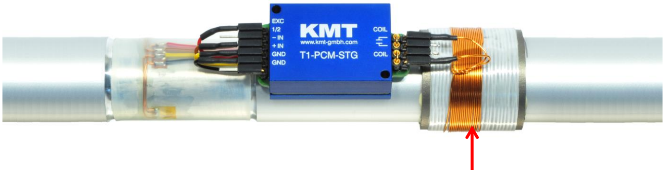
Coil, depends of shaft diameter 5-18 windings of 0.5 CUL wire
