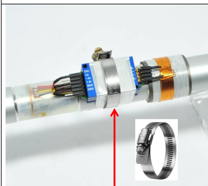
We recommend add. use a steel hose clamps for final fixing!!
