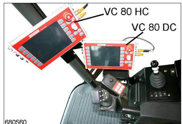
Fig. 4: Operator cabin with displays
